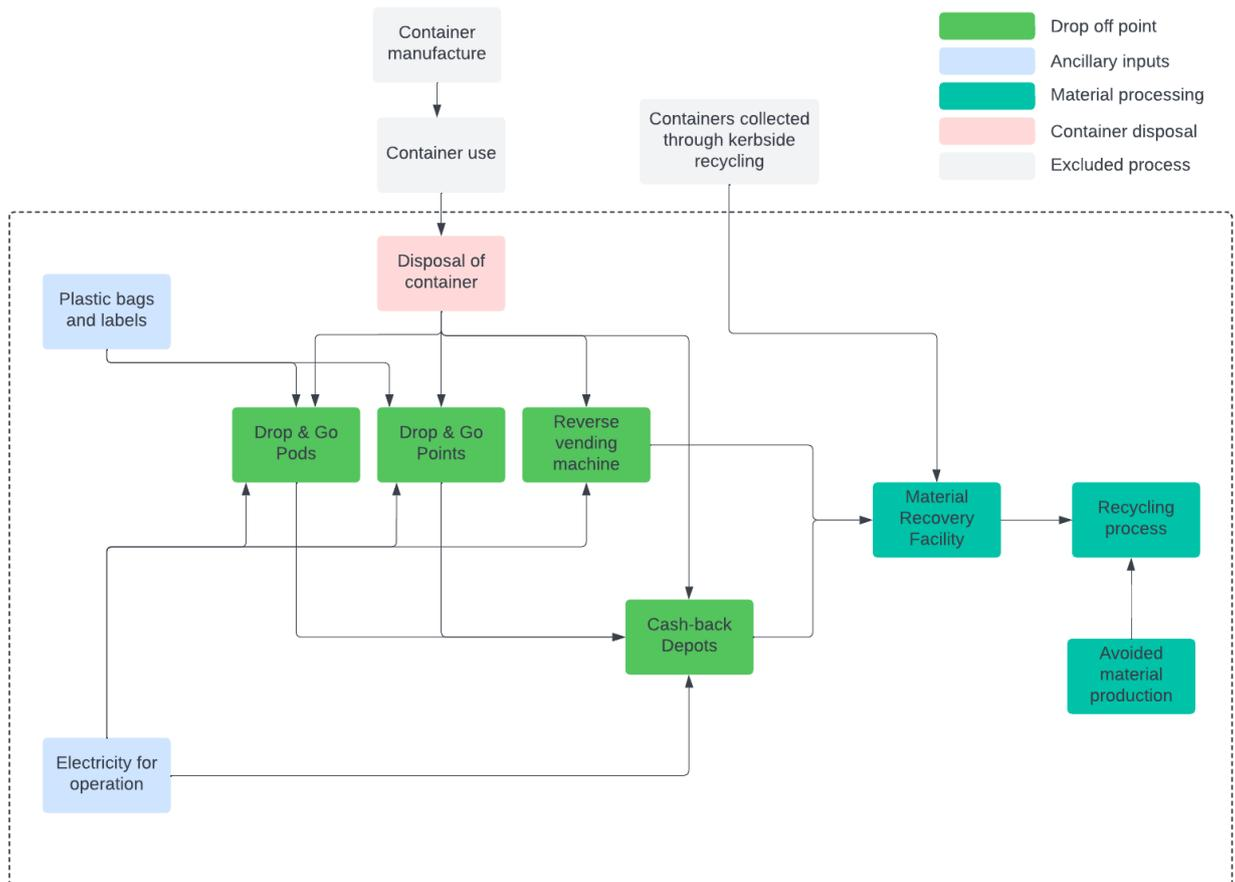
**Figure 4 Container deposit system boundary schematic**
