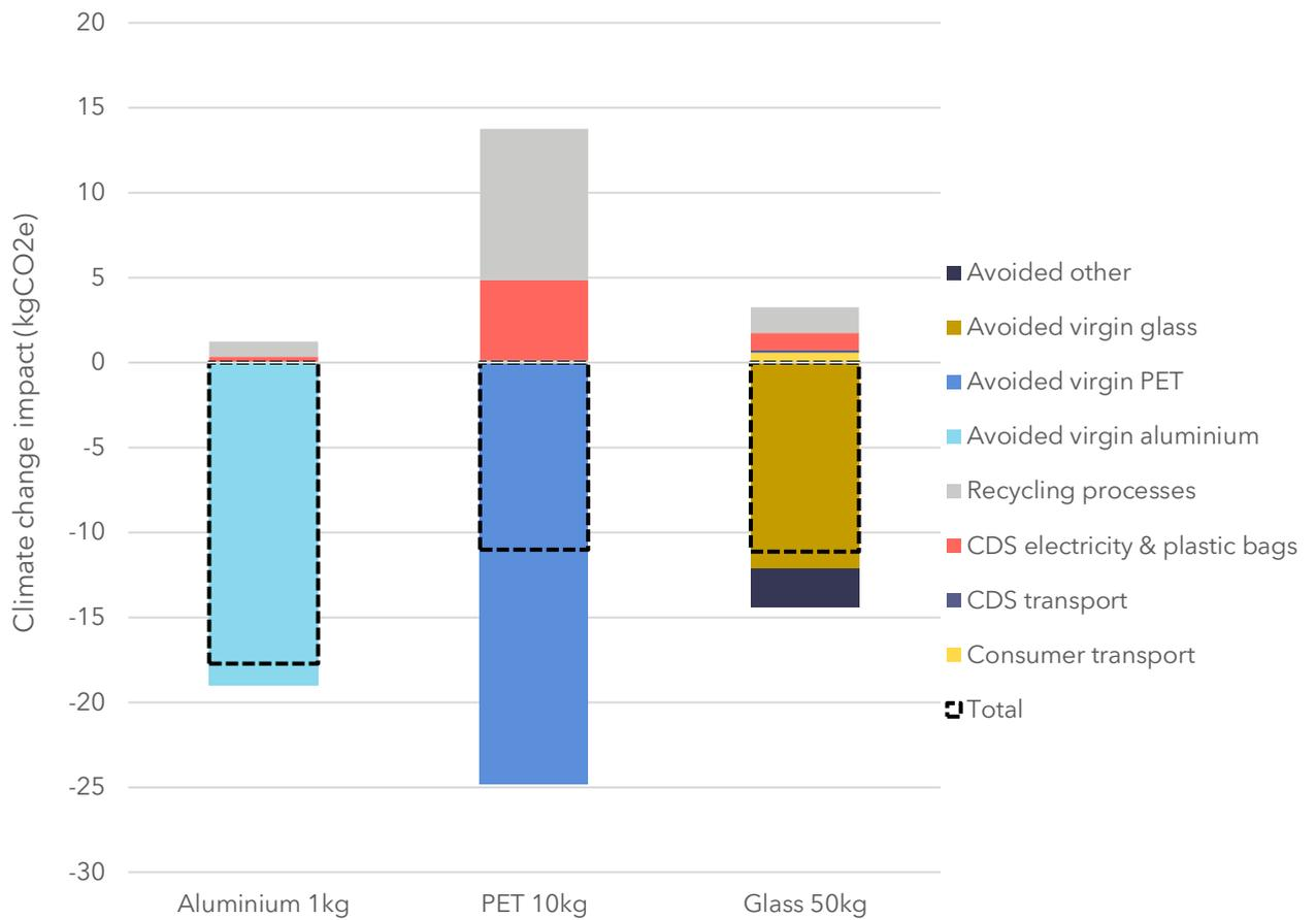
**Figure 9 Climate change impacts in kg CO<sub>2</sub>e per kg of aluminium, 10 kg of PET and 50kg of glass material entering CDS**
